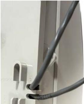
3. Align the remote module backplate with the mounting screw holes. Verify the Itron logo is not upside down.
