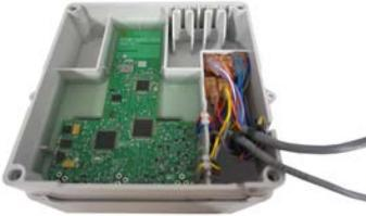
2. Route the register cable through the bottom backplate cable cutout and leak sensor cable through the top backplate cable cutout.
