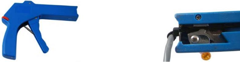
**Note:** If your cable tie gun is equipped with a dial to set the tightening pressure, set the pressure to ensure the cable tie is secure on the lead wire. After installation, the cable tie must not move on the register or secondary lead wire.
